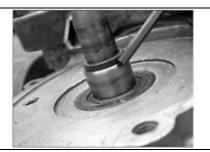
Correct. Note fit of spacer on shaft.
